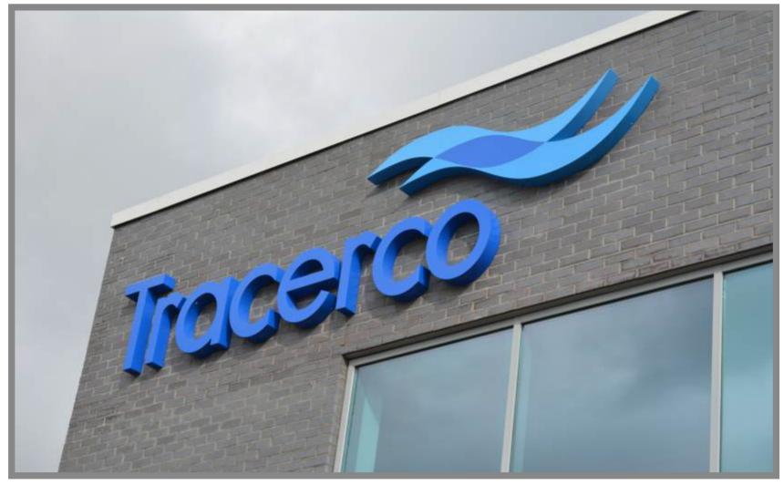
Fabricated letters are frequently used in shopping centres, the letters can be built to almost any depth and are often illuminated with LED'S internally and can generate many different lighting effects.
